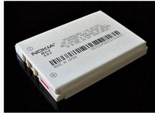
An example of a Li-ion battery (used on the Nokia 3310 mobile phone)
